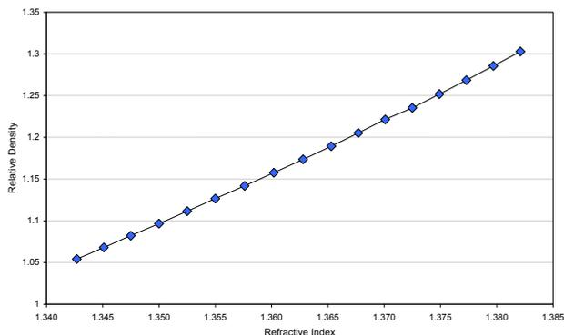
Fig. 1. Relation between density and refractive index of the electrolyte in lead acid batteries.
