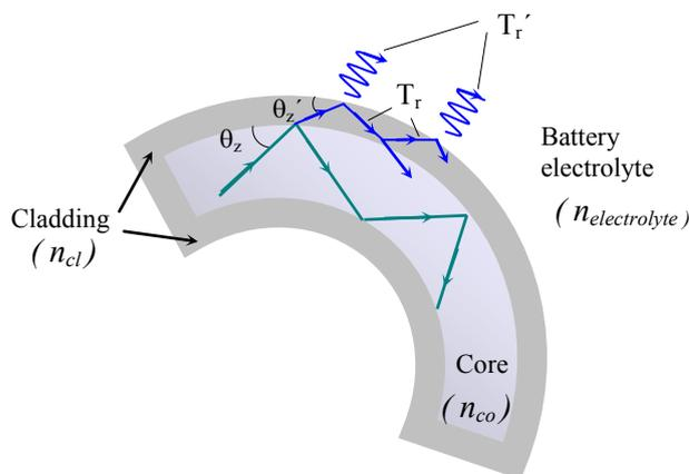
Fig. 3. Optical power losses in the bended zone of the fiber (sensitive zone).
