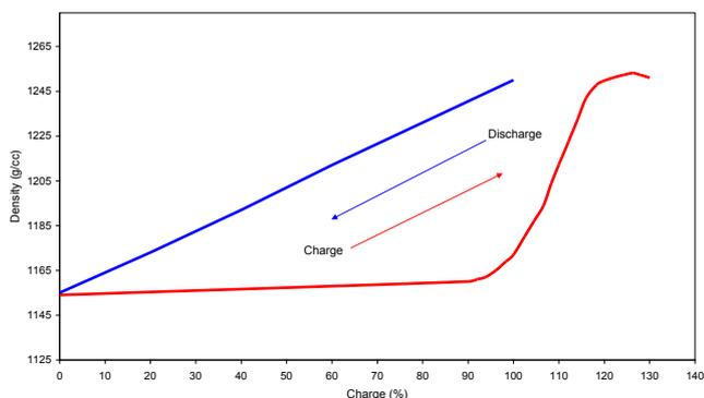
Fig. 2. Variation of density at the top of the battery during the charge-discharge process.
