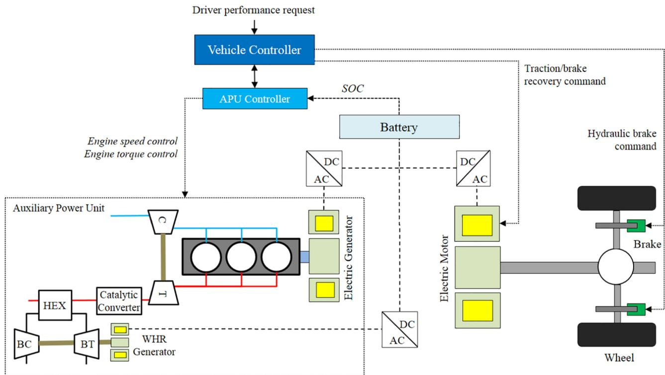
Fig. 1. Configuration of a simple Brayton WHR system on ICE coupled to a series hybrid electric vehicle.
