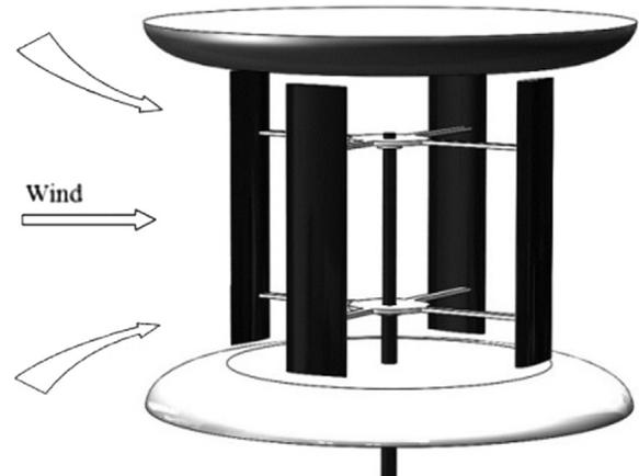
Fig. 1. Concept of WGD set top and bottom of the rotor.
