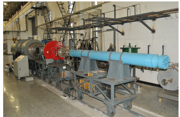
Fig. 1. CARDC's 3 kg/s pulse combustion wind tunnel.
