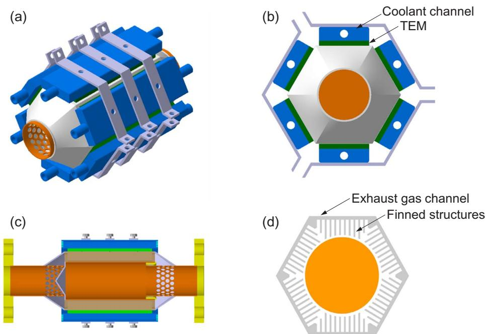
Fig. 1. Schematic diagrams of present hexagonal TEG: (a) isometric view, (b) front view, (c) cross-sectional side view of TEG, and (d) cross-sectional front view of exhaust gas channel.
