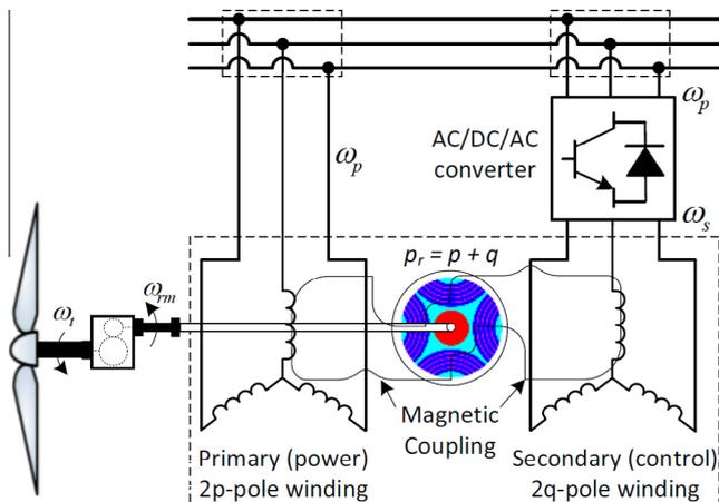
Fig. 1. A conceptual diagram of the BDFRG based wind energy conversion system (WECS).
