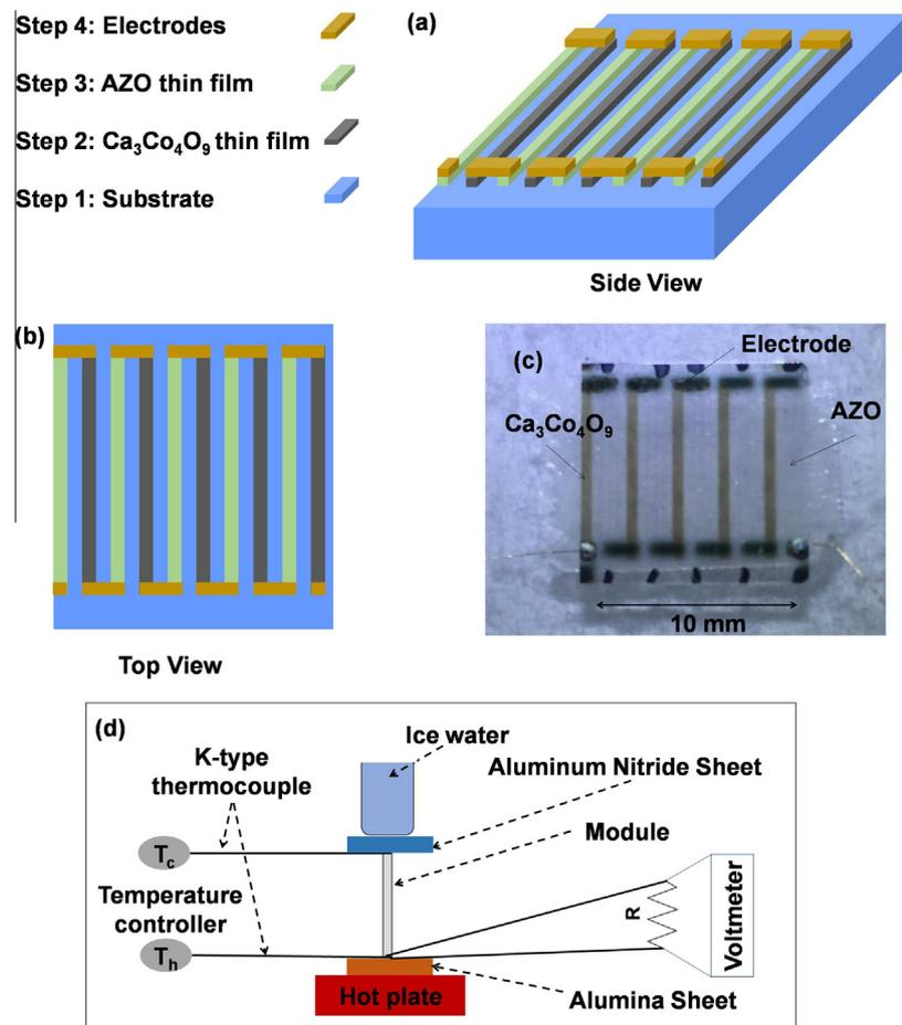
Fig. 1. (a) 3D sketch of the thin film module with sequence of thin films and electrodes deposition; (b) schematic top view of the module and (c) photograph of the module after fabrication of thin films legs and gold contacts; (d) schematic of module testing set-up with a load resistor ( $R$ ).
