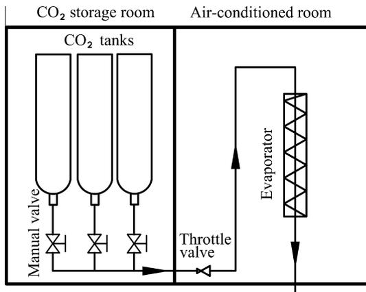
**Fig. 1.** CO<sub>2</sub> open refrigeration system. The arrows represent the flow direction of CO<sub>2</sub>.
