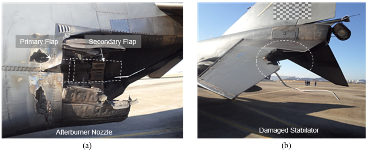
Fig. 2. (a) Damaged afterburner nozzle components and (b) stabilator.
