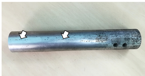
Fig. 1. The image of the failed valve stem showing corrosion attack and axial cracks (indicated by arrows) at several locations.
