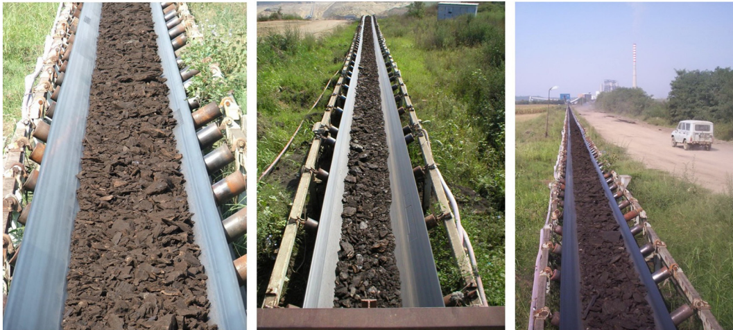
Fig. 1. Example of a rubber-textile conveyor belt used in real operation.
