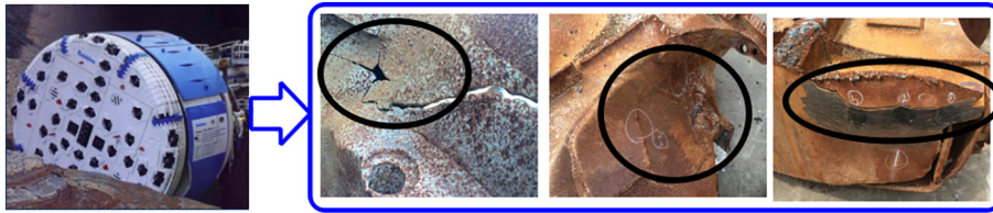
Fig. 1. Multiple cracks failure of TBM cutterhead.
