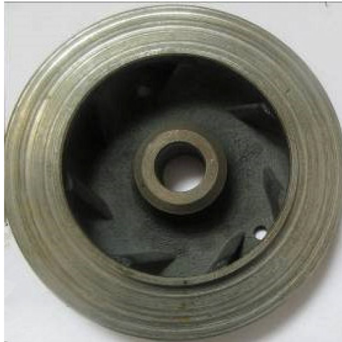
Fig. 1. Wear scar of impeller.
