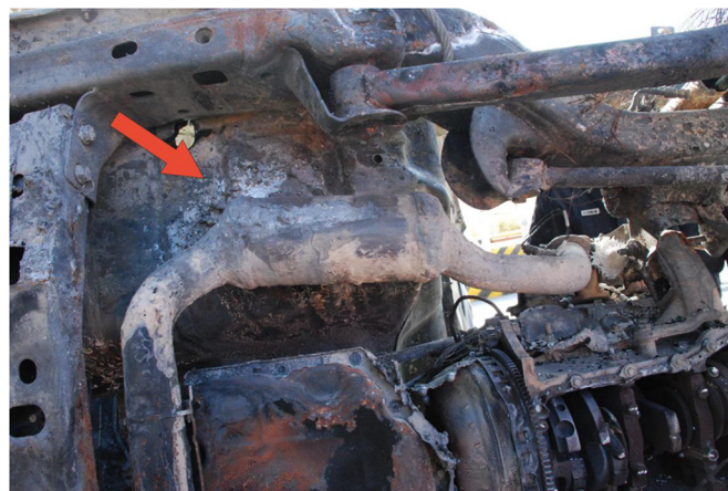
Fig. 3. Area of origin of fire exhibits significantly more damage and color change compared with the others.
