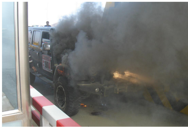
Fig. 2. First picture taken after the fire indicating the fire origin.
