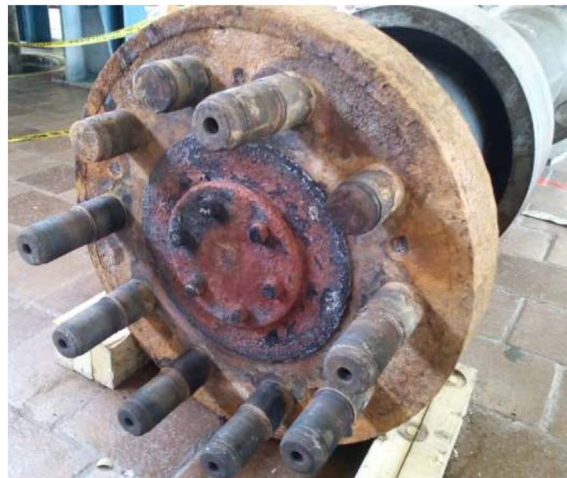
Fig. 2. Turbine shaft with the bolts after turbine removal.
