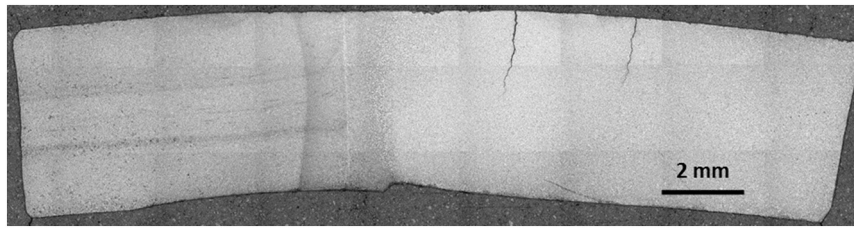
Fig. 1. X42 pipe transverse view showing weld and typical straight stress corrosion cracks.
