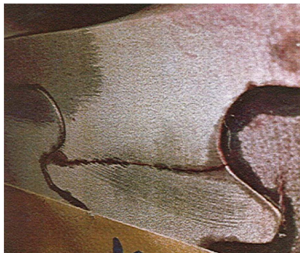
Fig. 1. View of the blade root with crack.
