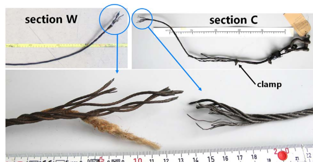
Fig. 2. Winch rope sections W and C with fracture brushes (circles). See also Supp. 3. Winch rope sections W and C with fracture brushes (circles). See also Supp. 3.
