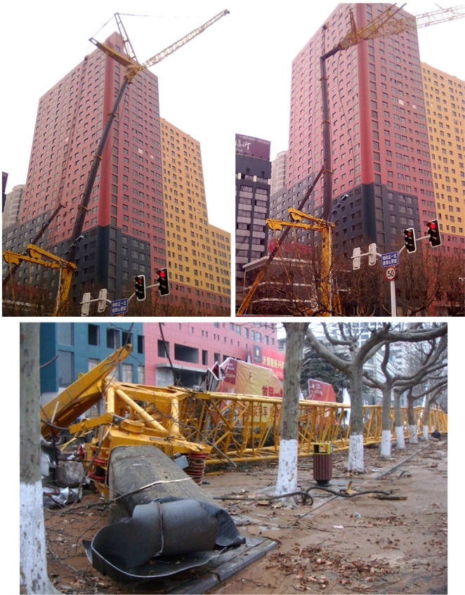
Fig. 1. Failure of all-terrain crane telescopic boom.
