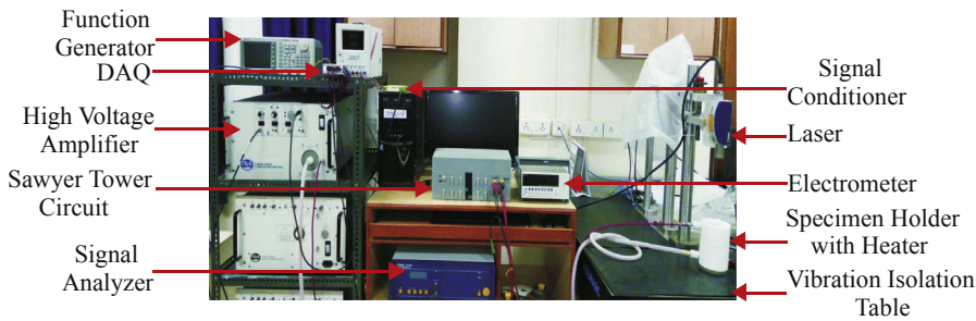
Fig. 1. Photograph showing the experimental setup to measure rate and temperature dependent electric displacement and strain under stress-free cyclic electrical loading of 1–3 piezocomposite.
