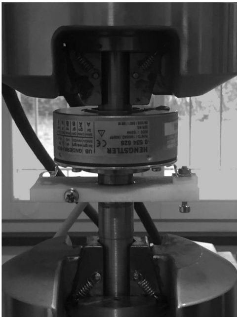
Fig. 2. Picture of the specimen fixed to the testing machine, including the twist angle measurement system.
