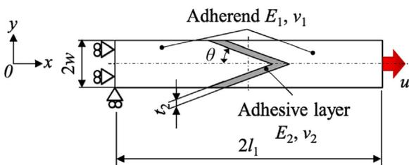
Fig. 1. A DSJ model with boundary conditions.
