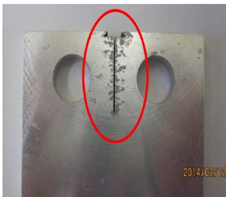
Fig. 1. C(T) specimen after two months outdoor exposure at Daytona Beach.
