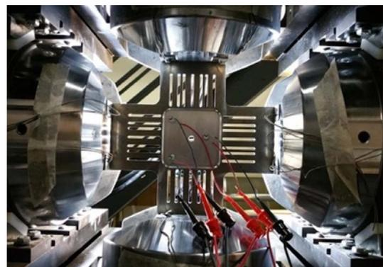
Fig. 1. Cruciform specimen in biaxial test frame.
