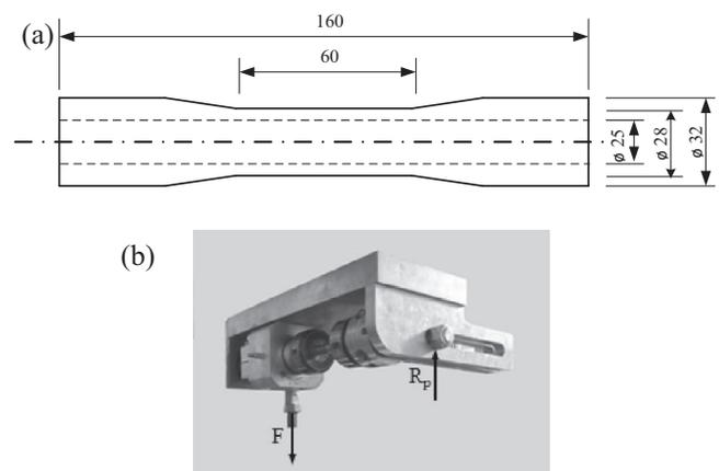
Fig. 2. Specimens geometry and fatigue testing device. (a) Tubular specimen. (b) Bending/torsion testing device.
