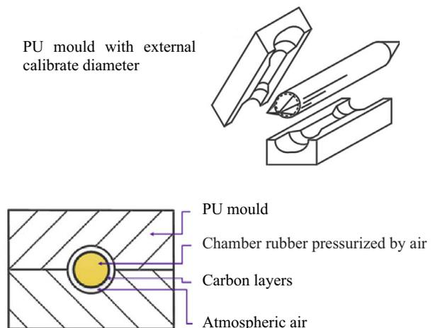
Fig. 1. Schematic view of the moulding process.
