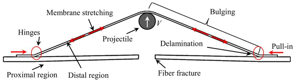
Fig. 1. Schematic illustration of deformation and failure mechanisms of a UHMWPE cross-ply laminate impacted by a spherical projectile.
