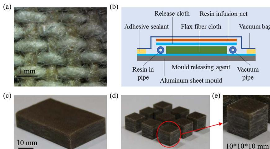
Fig. 1. Fabrication of laminated composites reinforced with (a) flax fiber weave based on (b) VARI. (c) Fabricated laminate, (d) tested samples, and (e) dimensions of a single cubic sample.
