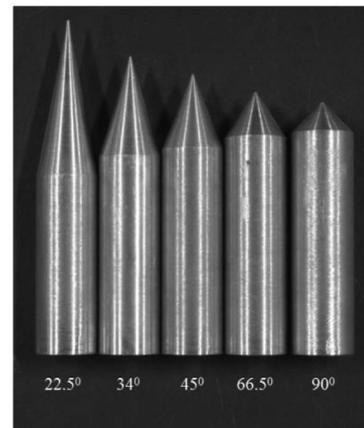
Fig. 2. Projectiles used in the current study before impact.
