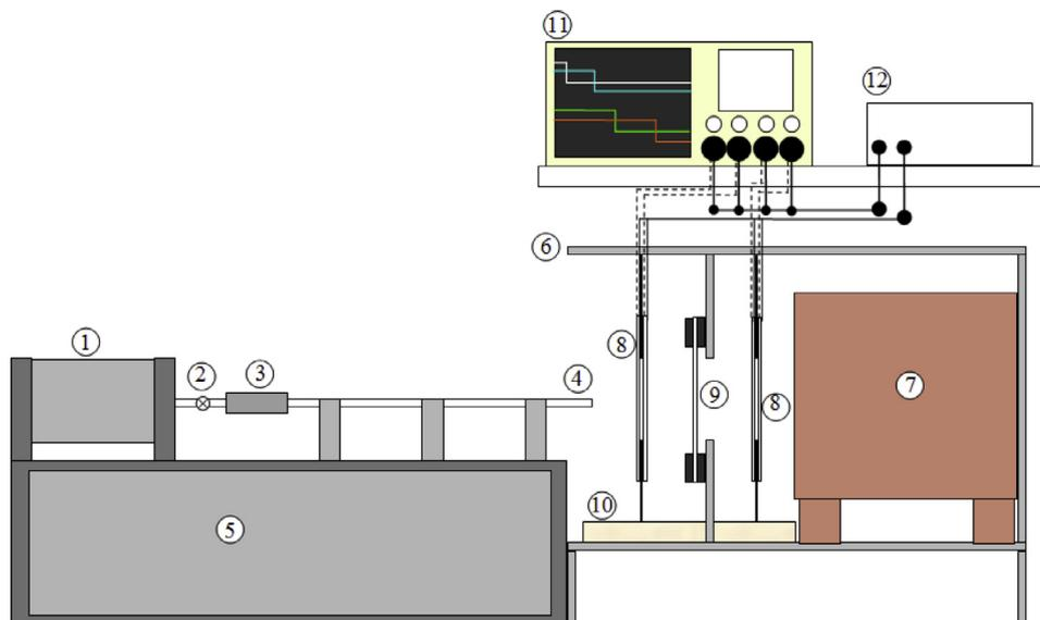
Fig. 1. Schematic representation of experimental setup ((1) Air cylinder, (2) Ball valve / Trigger, (3) Port for breech loading of projectile, (4) Barrel, (5) Machine tool bed, (6) Frame, (7) Projectile recovery box, (8) Foil set for velocity measurement, (9) Target, (10) Additional cushioning, (11) Oscilloscope, (12) Power supply and conditioning circuit).
