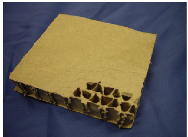
Fig. 1. Test sandwich panel, hat cushion.
