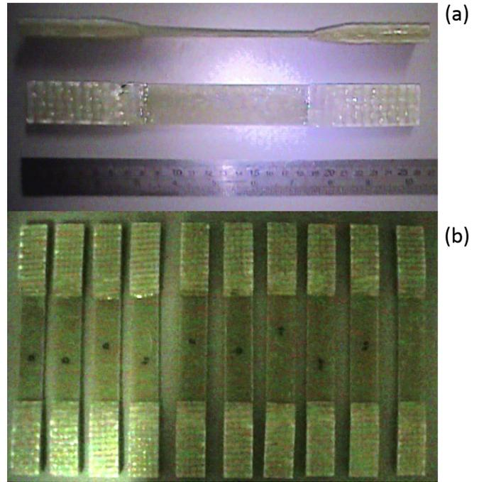
Fig. 3. Top and side view of tensile test specimen (a), tensile specimens with 0° and 90° (b).
