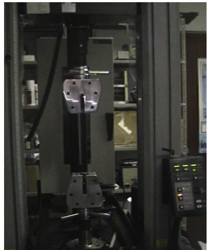
Fig. 4. INSTRON 5567 universal test machine.
