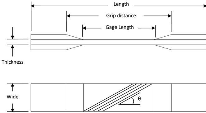
Fig. 1. Schematic views of tensile test specimen and dimensions.
