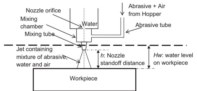
Fig. 1. Schematic of submerged abrasive water jet. Not to scale.
