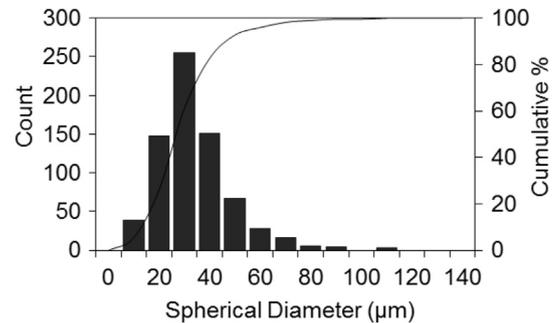
Fig. 2. Particle size distribution of garnet abrasive. Curve gives cumulative percent.
