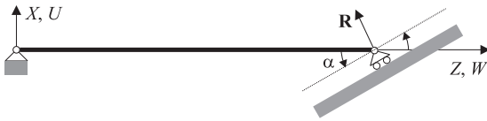
Fig. 1. The considered mechanical model. The slope is \beta = \tan \alpha .
