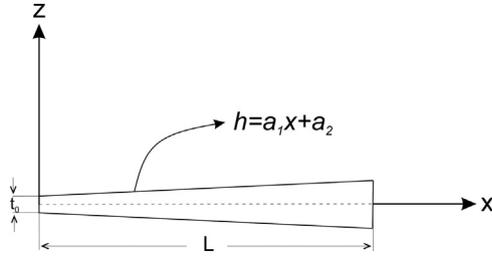
Fig. 1. Tapered beam in the Cartesian coordinate system.
