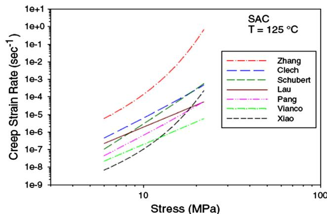
Fig. 1. (3–4) orders of magnitude variability observed in steady state secondary creep strain rates in SAC305 solder alloy tested at 125 °C (Ma and Suhling, 2009).
