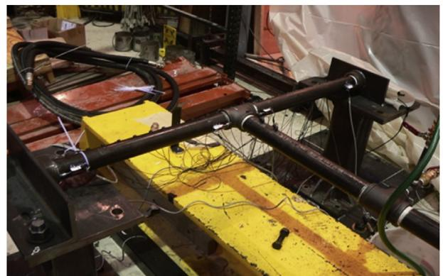
Fig. 1. Test setup for experiments on threaded Tee-joints conducted at UB.
