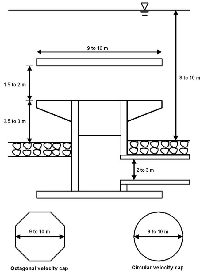
Fig. 1. Typical intake structure.
