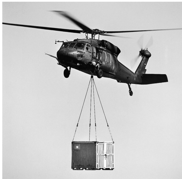
Fig. 1. Blackhawk with CONEX underslung load (Raz et al. (2008)).
