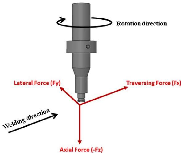
Fig. 2. Schematic of the defined generated forces directions during FSW process.
