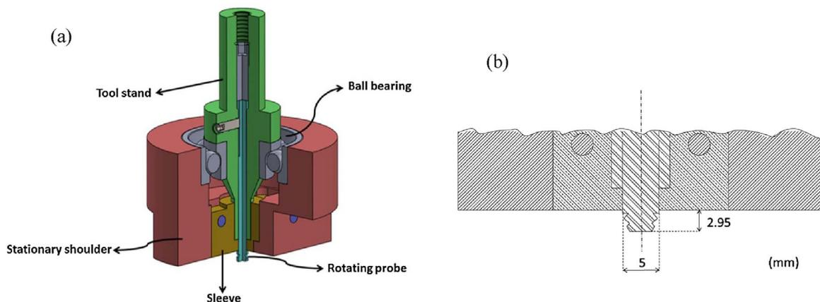
Fig. 3. FSW tool 3D CAD model (a); section view of the probe (b).
