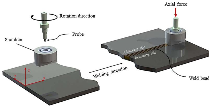
Fig. 1. Schematic of FSW butt-joint using stationary shoulder.
