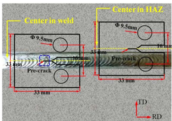
Fig. 2. Dimensions of compact tension specimen and schematically illustration of sampling locations.
