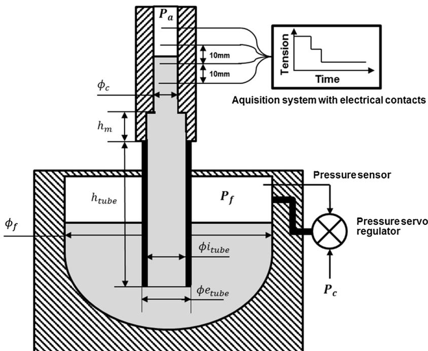
Fig. 1. Vertical cross section view of the Low-pressure casting system and instrumented sand mold.
