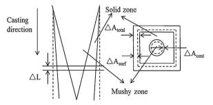
Fig. 2. Schematic diagram of the solidification model.
