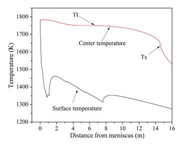
Fig. 1. Predicted temperature at the surface and the center of billet.
