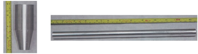
Fig. 1. Al sleeve (left) and Mg core rod (right). Billet components prior to composite billet assembly.
