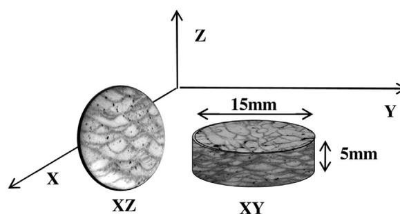
Fig. 2. schematic representation of the directions of the production of test specimens.
