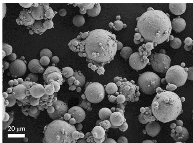
Fig. 1. SEM image of the AlSi10Mg powders employed in this study.
