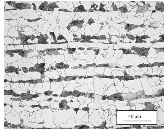
Fig. 1. Microstructure of the material before heating (Ferrite: White, Pearlite: Black).
