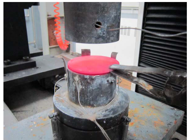
Fig. 3. Experiment setup showing the specimen and thermocouple wiring.
