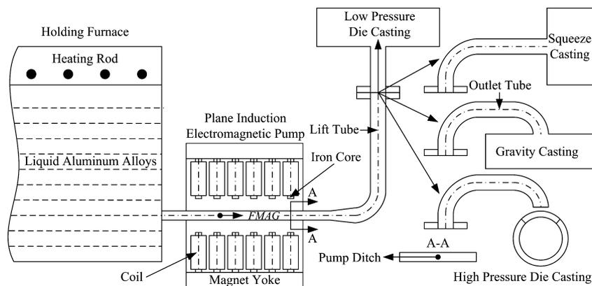
Fig. 1. Schematic diagram of the EMT process of liquid aluminum alloys during casting.
