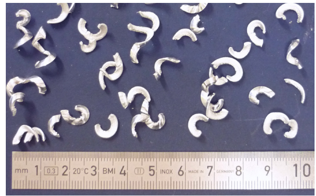
Fig. 1. Produced AA6060 aluminum alloy machining chips used in this study.
