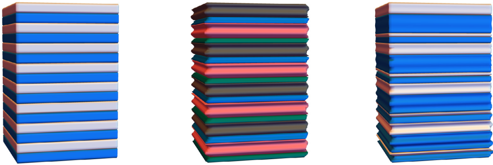
Fig. 1. Laminates with different periodic cells. The band structure describes which frequency bands are of propagating waves (middle laminate), and which frequencies belong to gaps of decaying waves (right laminate), depending on the periodic cell composition. In this work, we unveil a generalized object that encapsulates the infinite band structures of all multiphase laminates impinged by normal waves, independently of the specific composition.
