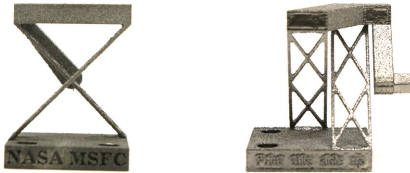
(a) Front view of cross-axis flexural pivot (CAFP) made with lattice flexures. (b) Side view of lattice-flexured CAFP.
