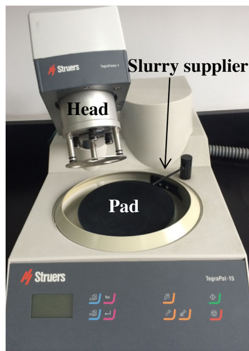
Fig. 1. Photograph of the TegraForce-1/TrgraPol-15 polisher.
